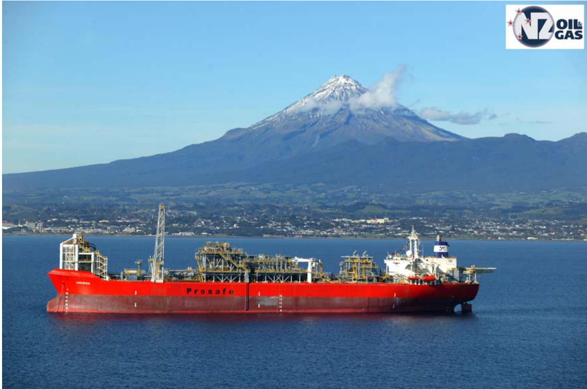
Umuroa FPSO (Floating Production, Storage, & Offloading) vessel to be used for the Tui oil production in offshore Taranaki Basin with Mt Taranaki in the background.
